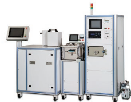
Ex) Combination with SAL3000Plus ALD Outer dimension : W2014×D1040×H1827 (mm)
